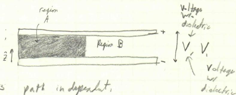
We know that Voltage is path independent, so the Voltage across Region B is the same as across Region A, namely,  $V_1$ . We know the dielectric's Voltage is reduced by  $\epsilon_r$  so
